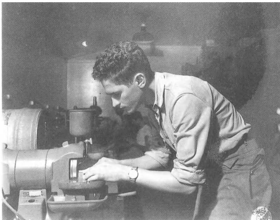
11. A Signal Corps technician carries out edge grinding on a set of quartz blanks. Philippines, 1945. SC235280
