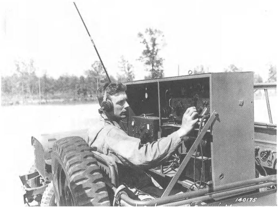
17. Radio operator seen at his radio that is permanently mounted in a jeep. SC140175
