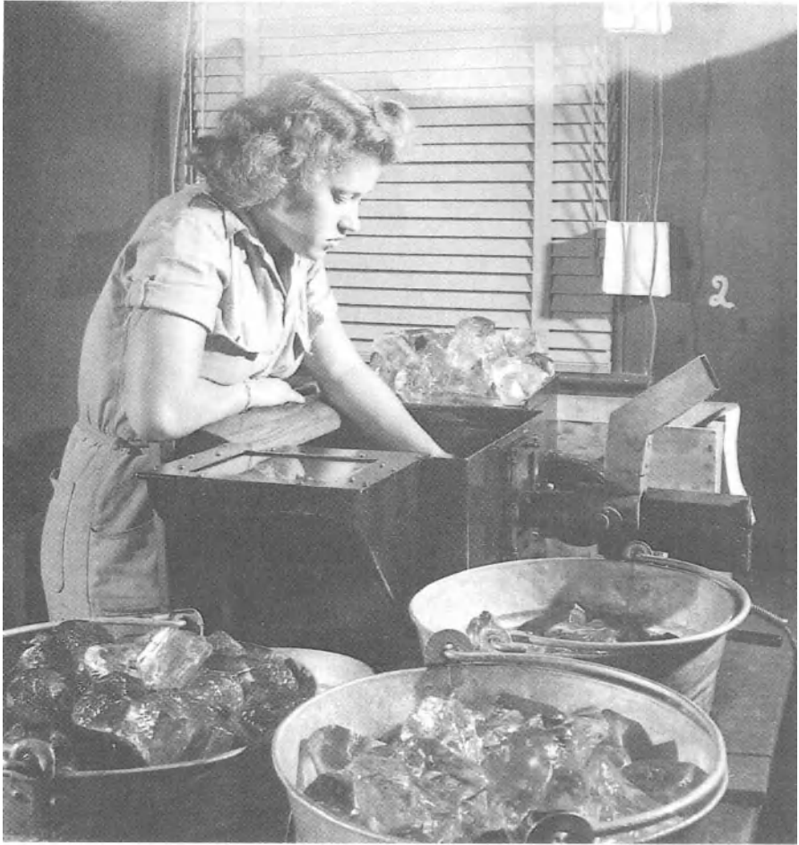
4. Checking quartz crystals for internal flaws utilizing a mineral oil bath. Rio de Janeiro, Brazil. 169-GA-6B-2
