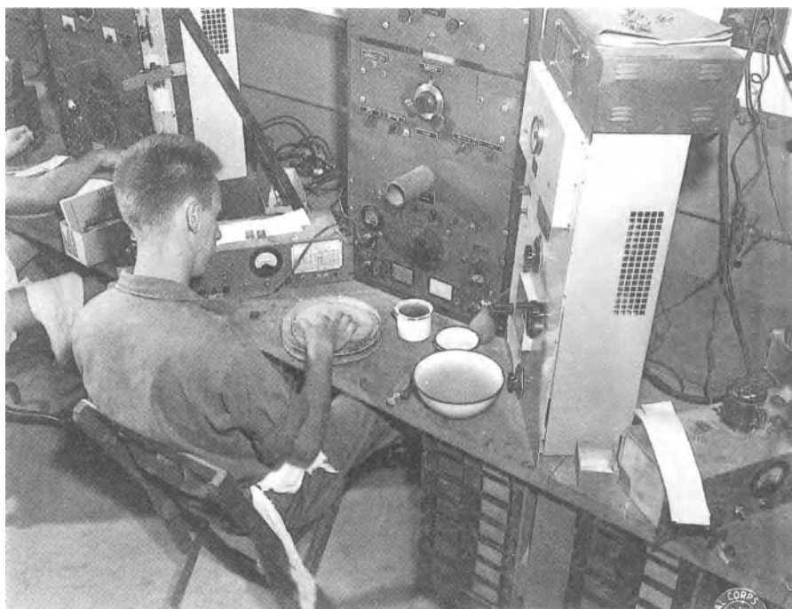
12. Hand grinding, the final stage of the production process, is carried out by a Signal Corps technician. Philippines, 1945. SC235279
