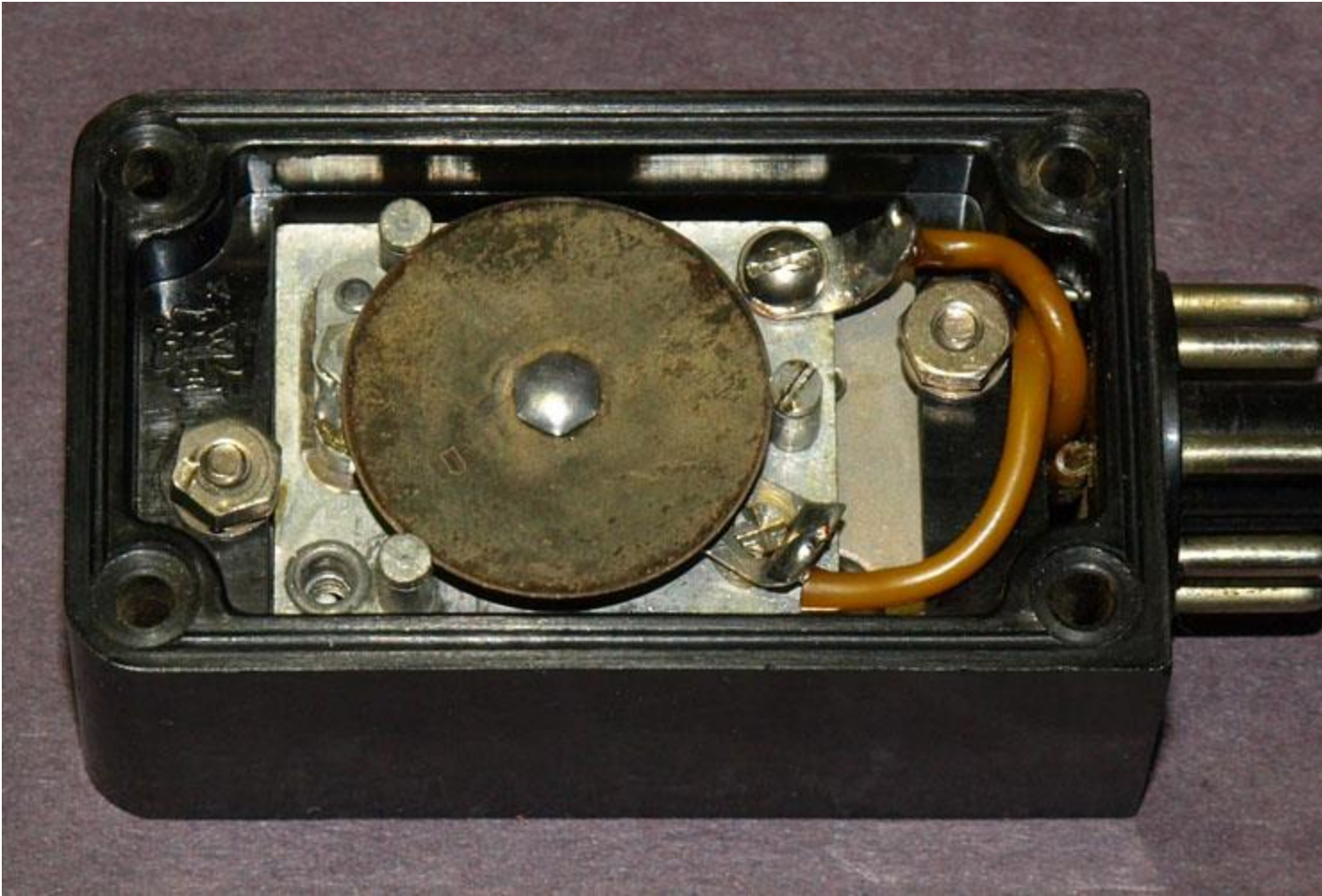
Cover open to show the temperature sensor. The round disk is temperature sensitive pushing on a contact switch below it. This contact is no longer part of the circuit. One screw is shown removed (bottom left) which contained a grounding clip for the metal case
