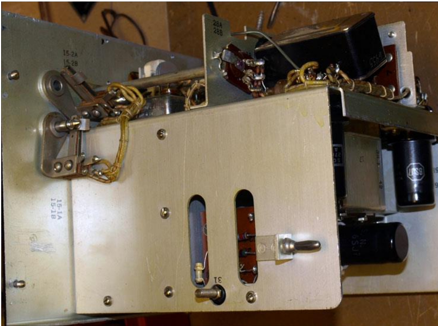
Docking adapters on the other side (ground on the right, antenna on the left).
