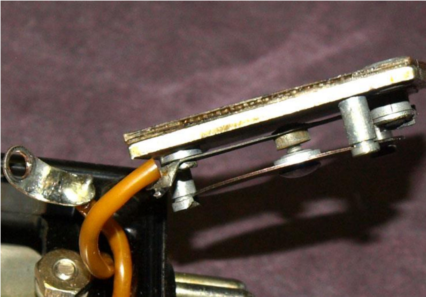
Relay in the closed position (this is the normal position). Mica insulator can be seen facing up.
