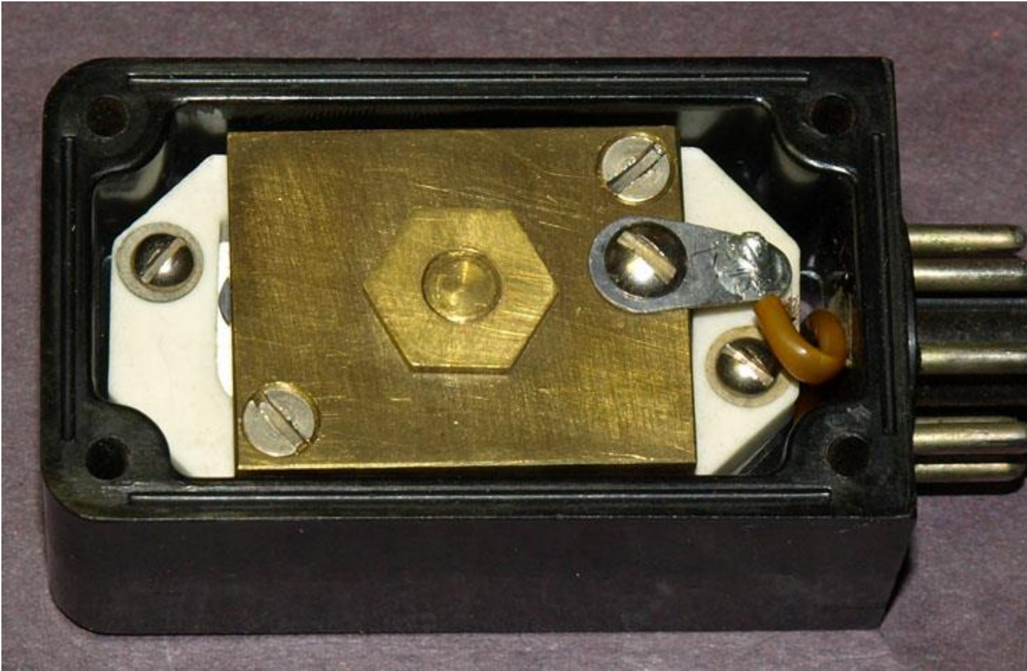
Cover open to show the contact plate for the crystal.
