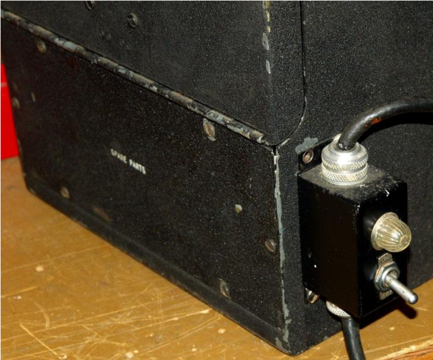
Power switch mounted on the side of the cabinet.
