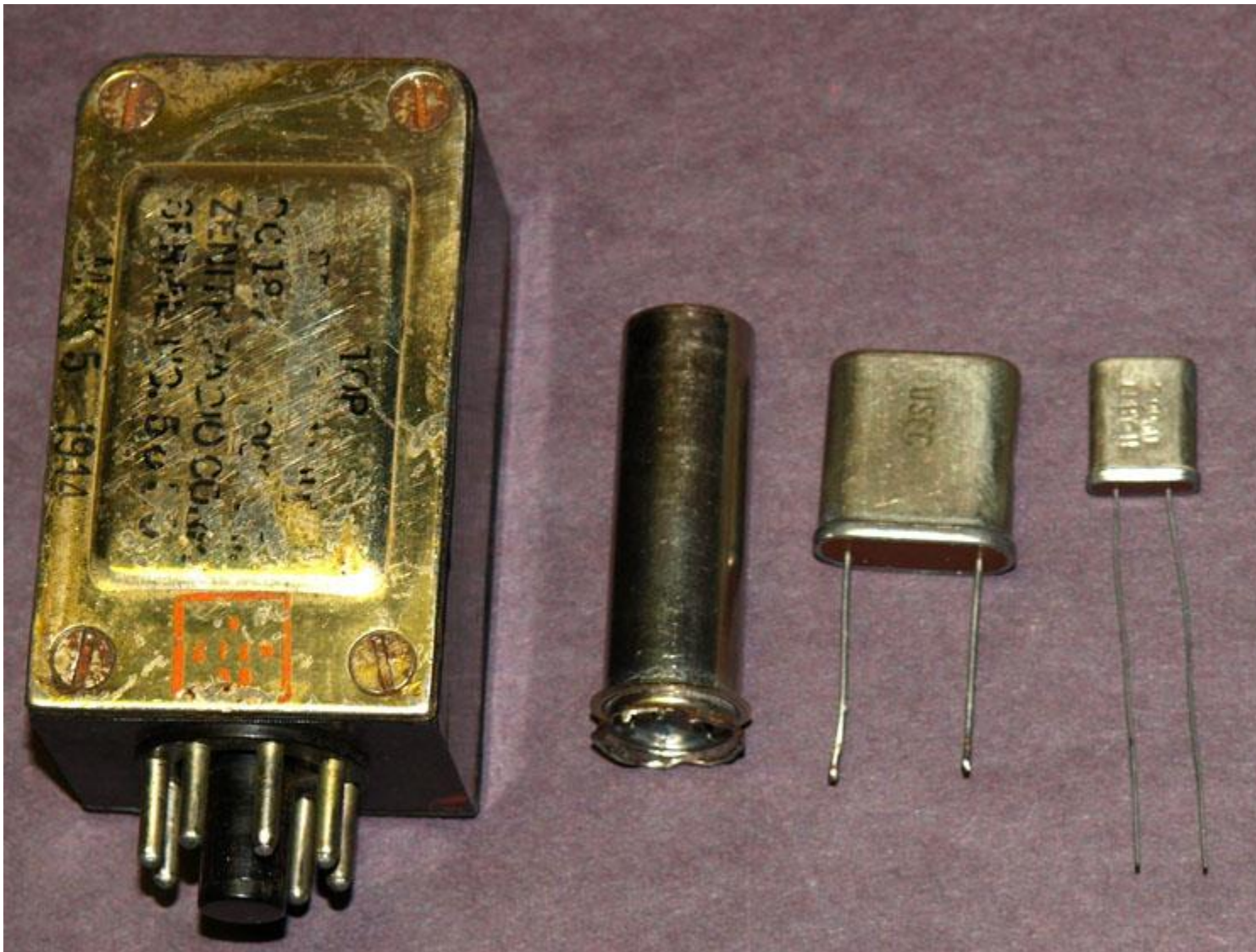
Comparison of several crystal packages (the smaller, the more modern)!
