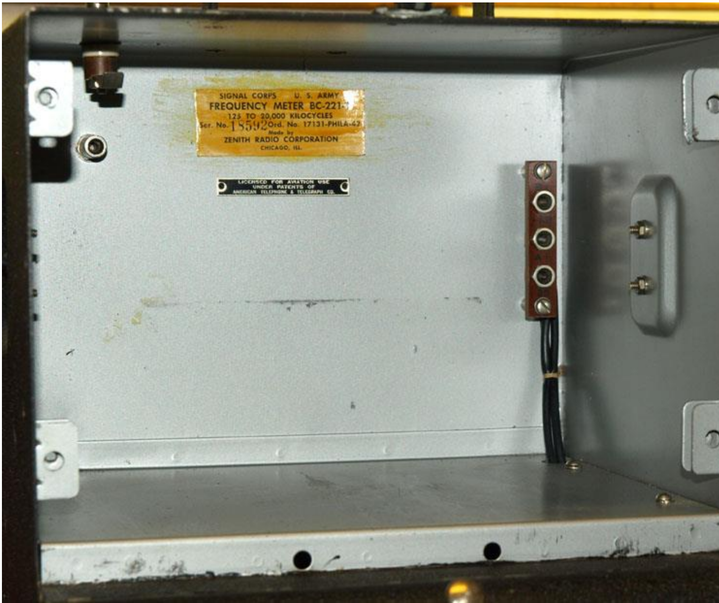
The electronics can be pulled out of the cabinet. Note the docking adapters in the back.
