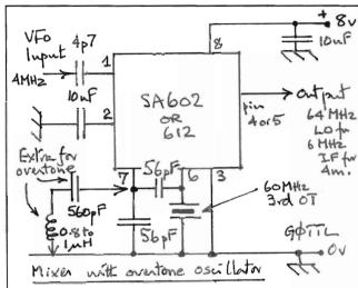
I've done a few tests with overtone crystals I had to hand and it does work well, the highest frequency I've tried so far was 120 MHz using a 5<sup>th</sup> overtone. I'm waiting now for the 60 MHz components to arrive and then I'll make a proper start on the VHF project. Watch this space!
