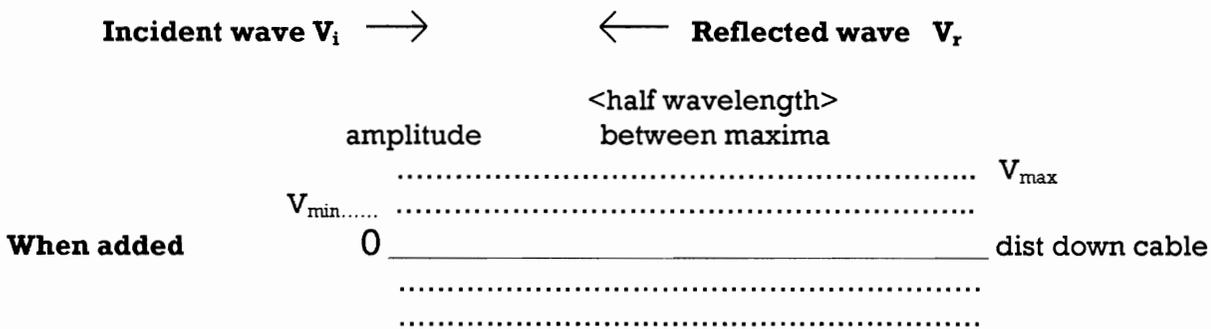
**VSWR =  $V_{max}/V_{min}$**  ← **This is the definition**  $V_{max} = V_i + V_r$  and  $V_{min} = V_i - V_r$
