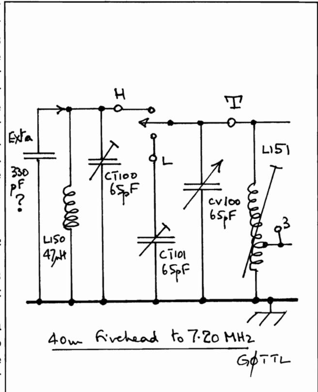
That's it, you should now be able to tune right up and down all of 40M. You might need to adjust the value of the 330 pF capacitor, if on the high switch setting the VFO frequency is too high, increase the capacitance or vice versa if it's too low. You shouldn't need to adjust the PA or band pass filters. Tuning wise it seems to be quite linear and has not affected stability in any way.
