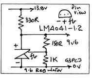
rig's 9.6 volts. I have some of the reference chips (or extra 317Ls) at 50p plus 50p postage in stamps. Supply range A reluctance to work properly on over 15 volts on transmit is due to restricted bias conditions around TR306/7/8. I regret there is no easy cure except to stick to under 14.5 volts! If you wish to reduce the *minimum* voltage that the rig will work on, place 10K in parallel with R122.
