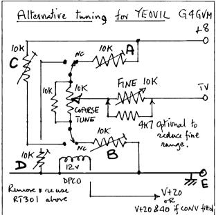
for a VFO frequency of 4990 KHz (RX at 13,990 KHz) with the tuning fully anticlockwise. Repeat the checks and adjustments remembering that if you have to adjust the TOKO slug then all will be affected. Eventually you can obtain the desired full swing on the two main bands and have them both tuning in the same direction.
