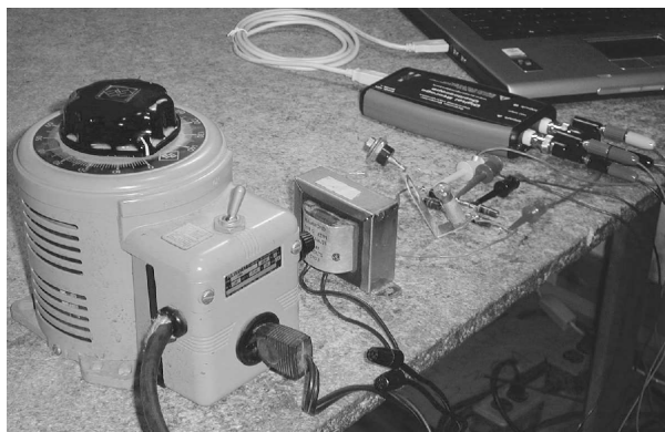
Figure 2: Line Voltage Autotransformer
