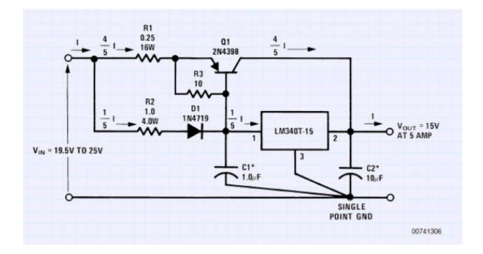
•The pass transistor base current cannot be ignored especially when several pass transistors are paralleled. The voltage drops across R1 and R2 in Figure 6 are NOT equal.
