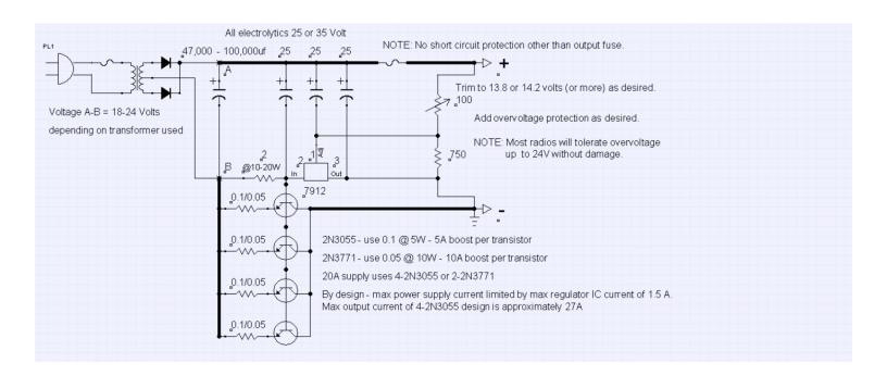
Do not remove the emitter resistors. The 0.1 ohm emitter resistors help compensate for DC gain variations among devices. The base currents will not be equal but collector currents will be nearly equal.
