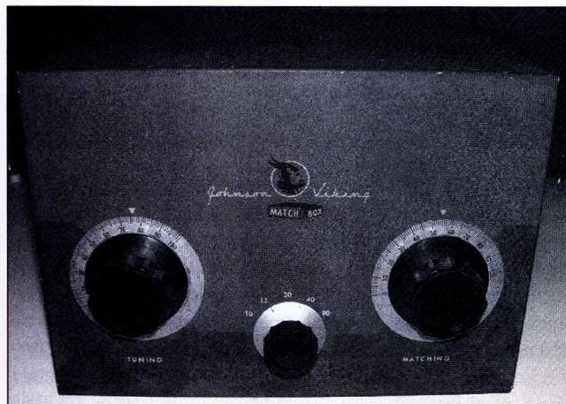
**Figure 3-7 — 1950's vintage E. F. Johnson Matchbox antenna tuner.**
