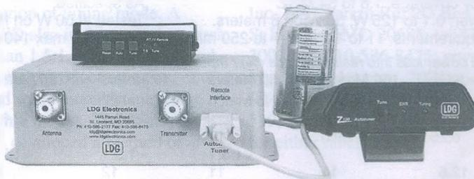
**Figure 14-18 — LDG RT-11 (left) with control box and Z-100. A 12 ounce beverage container provides scale.**
