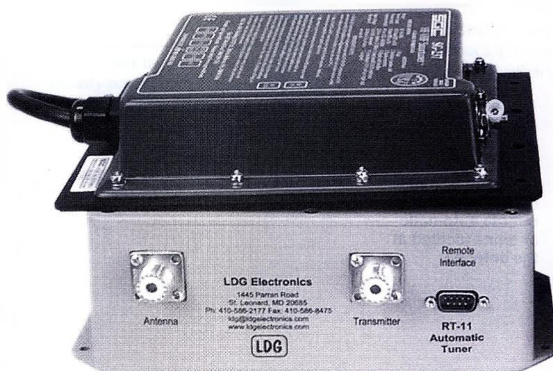
Automatic antenna tuners designed for remote mounting. On top, one from SGC, beneath a model from LDG.
