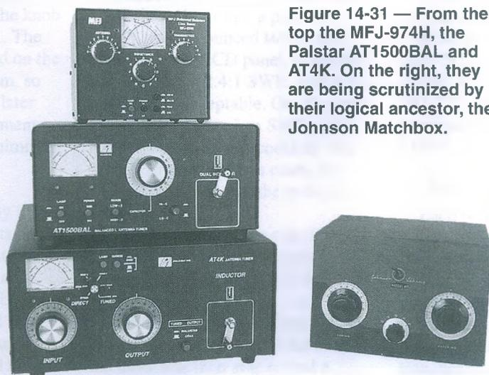
Figure 14-31 — From the top the MFJ-974H, the Palstar AT1500BAL and AT4K. On the right, they are being scrutinized by their logical ancestor, the Johnson Matchbox.
