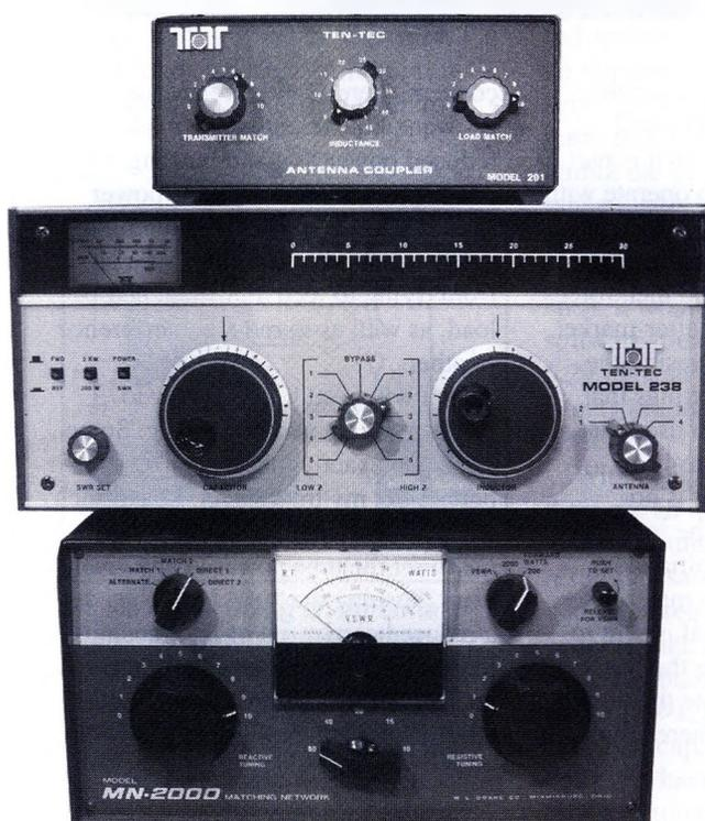
Tuning controls of three manual tuners. On top, a 100 W Pi-network, in the middle a 1500 W L network tuner and on the bottom a bandswitched 1000 W Pi-network tuner.
