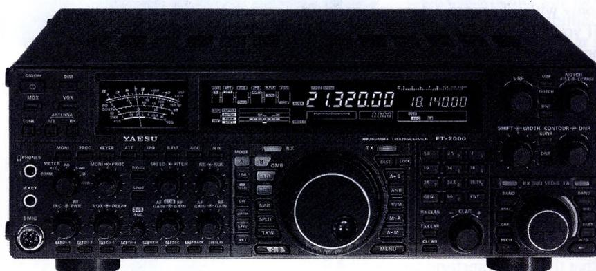
The Yaesu FT-2000 transceiver, one of many modern transceivers equipped with an automatic internal antenna tuner.
