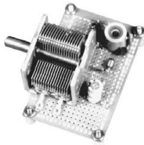
1-7 VFO circuit build on perftboard.
