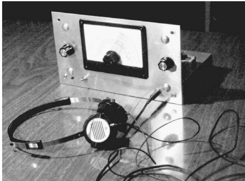
6-17 Photo of direct-conversion receiver.
