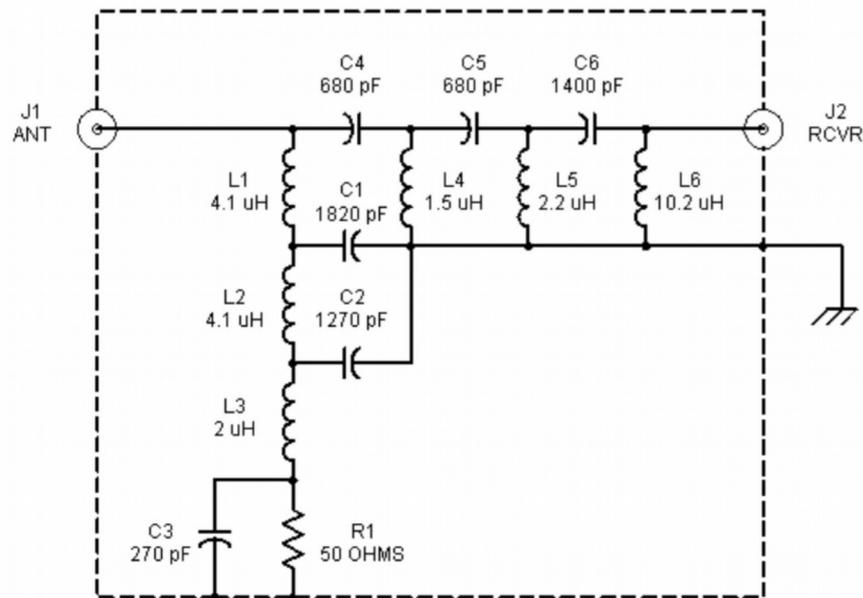
Joe's design features a low pass filter and a high pass filter, which, coupled together, block a full band of frequencies, the A.M. broadcast band. This allows our LF / VLF brethren to operate seamlessly VLF → LF → HF without having to exchange filter modules, a great idea if you're into HF and LF operating all at once!
