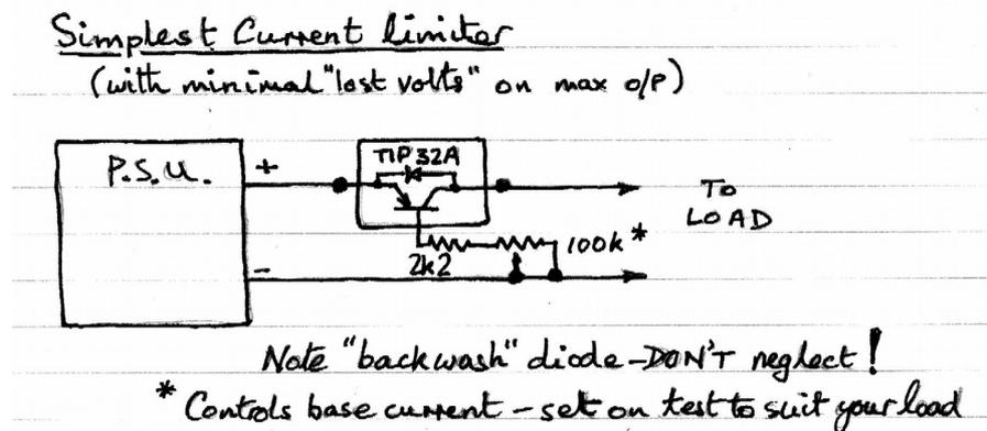
Below the current limit set by the base current (collector current =  $H_{fe} \times$  base current), the transistor feeds the circuit as a saturated switch, with only  $V_{ce-sat}$ , (0.2v or less) drop.
