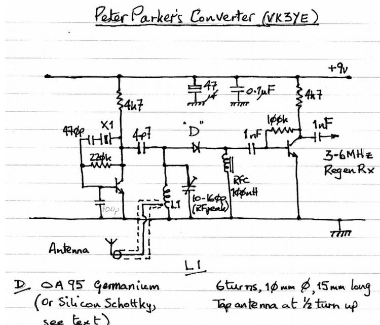
(Note: oscillator transistor base capacitor = 100pF )
