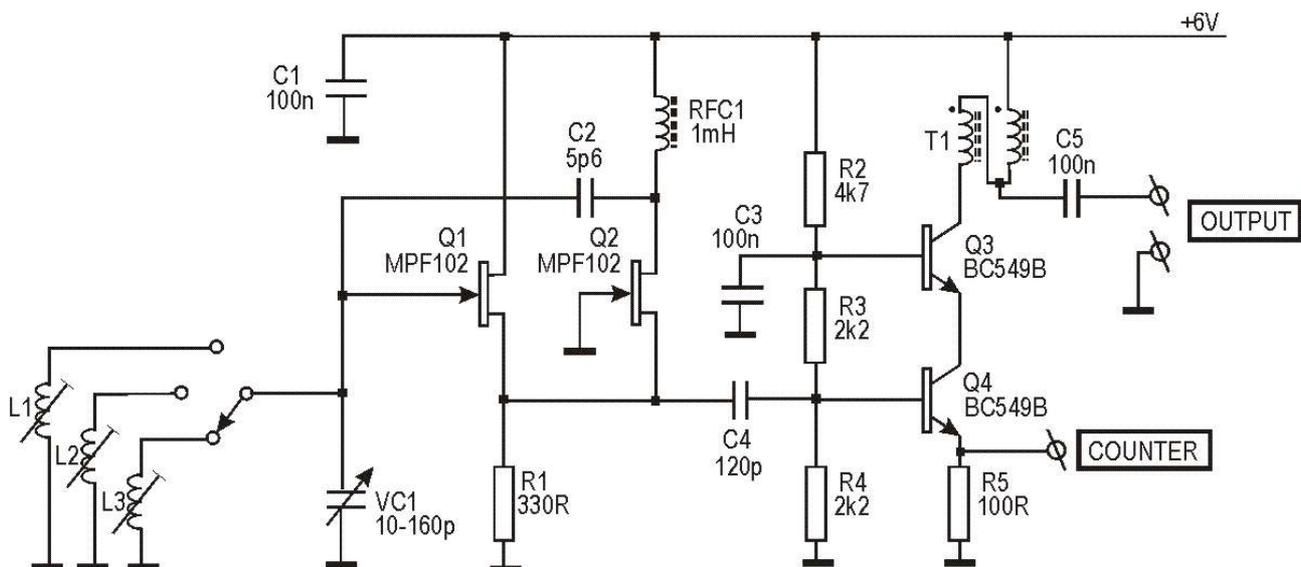
Andrew describes this as a signal generator, but those familiar with low voltage power output stages will recognise transformer T1 as being capable of a good few hundred milliwatts, if not a watt or so, of output. The design is simple, but elegantly sophisticated: much like quality commercial or professional equipment.
