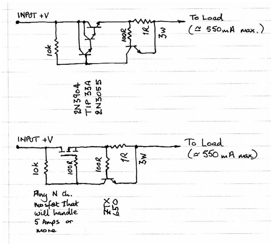
Note: you might need a 'backwash' diode on the Darlington circuit. You can set the maximum current with the 1R sense resistor:  $R=V/I$ , and  $V=V_{be}$  of the sense transistor (ZTX650). A sense resistor of  $0.47\Omega$  will give  $0.55v/0.47\Omega = 1.17$  Amps, for instance.
