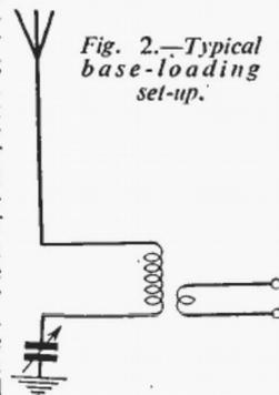
Fig. 2.—Typical base-loading set-up.
