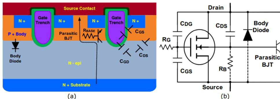
Illustrates clearly the parasitic devices created when constructing the device in silicon. Not perhaps as simple as you expected? And then you wonder why this thing 'hoots' at many MHz with a sniff of feedback and a few pF's and  $\mu$ H's?!
