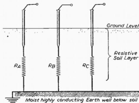
Fig. 1.—The arrangement necessary for measuring earth resistance.
