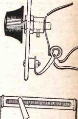
From an old Atwater-Kent model 40 radio, I removed the outside mounted potentiometer, using the case, knob and wiper. As shown, the wiper (of springy metal) moves across the turns of the voltage divider. The result is a smooth variation of resistance throughout the entire range. Adjust the wiper to make good contact yet little friction.
