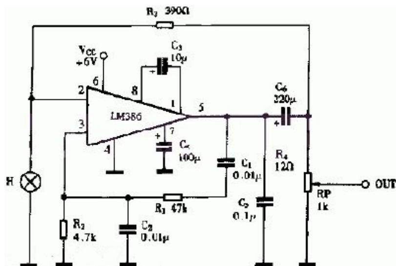
The arbitrary filament lamp (“H”) is usually a show stopper, but from experience an old Xmas tree bulb - or in fact any other filament lamp you can lay your hands on - or even a pair of back-to-back equal value zeners (3v3 or 4v7) plus a 1k series resistor. A bit of cut and try will get the job done.
