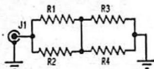
Wire resistors together as shown in schematic, then install in chassis box.
