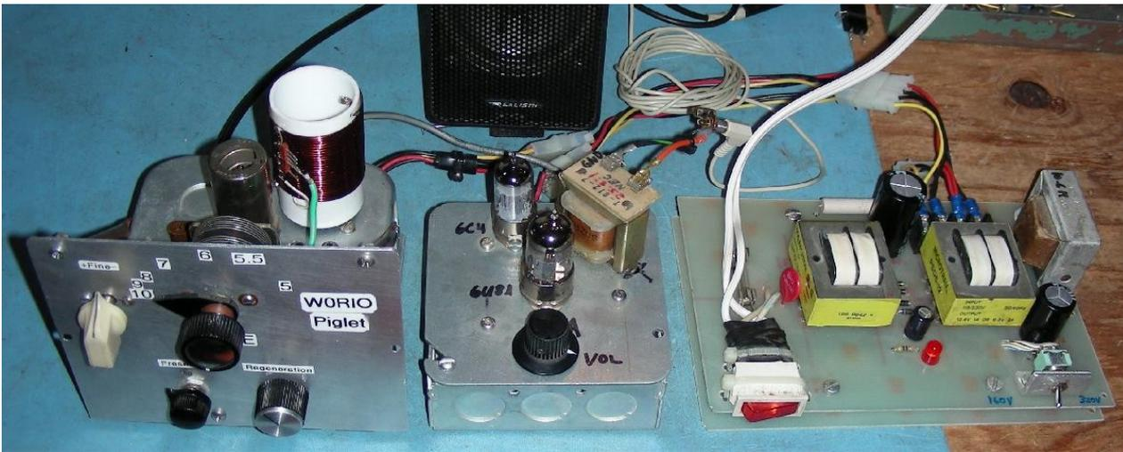
the design goals of the receiver was to be able to pick up both the 5Mhz and 10Mhz WWV time signals. When propagation conditions are good and the Piglet is connected to a good outdoor antenna, stations can be picked up across the entire tuning range of the receiver.
