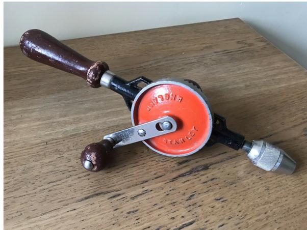
To mount the drill, you'll need a small vice - the suction based type is good - and this holds the hand drill by gripping the body beneath the large pinion wheel, thus putting the drill in a horizontal position. Some M4 steel bolts, 30mm long or more, with some M4 washers and an M4 wing nut for easy mounting of the sewing machine plastic bobbins in the chuck of the hand drill are used to grip and turn the bobbins.
