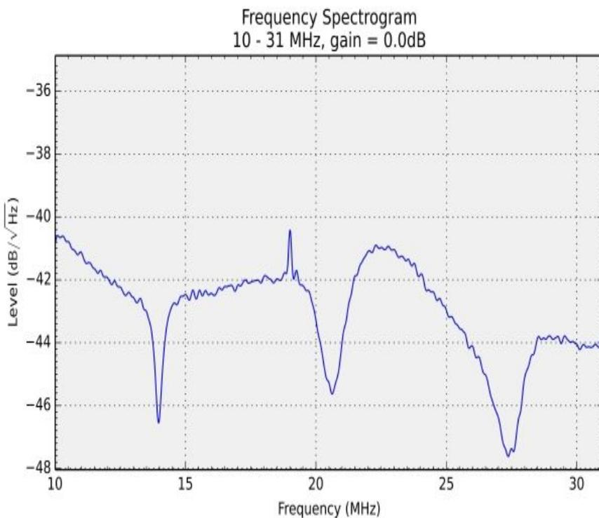
This is a more useful result and while I wouldn't claim this is a measuring device, it does fall into the category of an "indicating device" - and one that provides some indication of return loss relative for each of the three bands. I'm waiting for warmer weather to work out why my antenna has shifted "LF" a bit. My antenna analyser is telling me a similar story.
