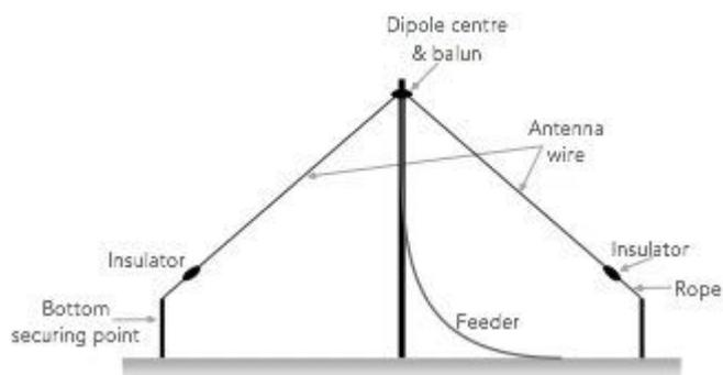
The inverted V dipole antenna has a number of advantages. One is that the maximum radiation from any antenna is from the points of high RF current, and a half-wave dipole has this maximum at its centre and for a few feet on either side of the feeder connections. Therefore it is best to make the centre of the dipole as high as possible.
