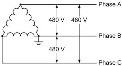
Used to reduce wiring costs by using a service cable with only two insulated conductors rather than the three insulated conductors used in a convention three phase service entrance.
