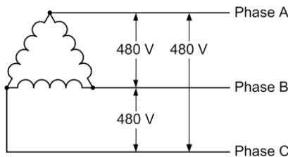
Used primarily in industrial facilities to provide power for three-phase motor loads, and in utility power distribution applications. Nominal service voltages of 240, 400, 480, 600, and higher are typical.
