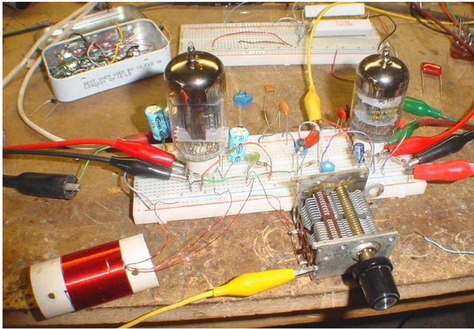
The radio was first built on a generic breadboard for experimenting. I soldered longer leads to the tube sockets so they could plug into the breadboard easily. The filament power for the two tubes were supplied by two separate low voltage bench supplies.
