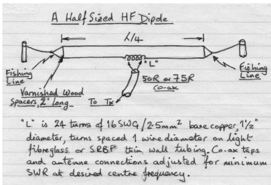
This half sized dipole gives excellent results, and makes matching easy (for cheap 75 ohm TV co-ax too!) with only one coil; but don't expect a wide bandwidth. The more you shorten an antenna, the "tighter" the resonance becomes; but for us A.M. nuts, with only one frequency slot in each band, the job's a good 'un! Keep the wires well separated, as high RF potentials exist along the wires.
