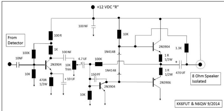
Figure 2—Audio amplifier schematic.
