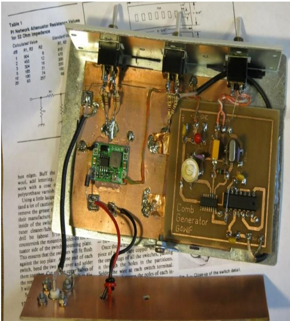
The small (left hand side) printed circuit board which the red and black power leads attach to is a very inexpensive switched mode "buck converter". This takes the 12 volt input and provides the 5 volt supply to the generator. There is an idiot diode in the supply in the event of one of those senior moments when the leads get reversed.
