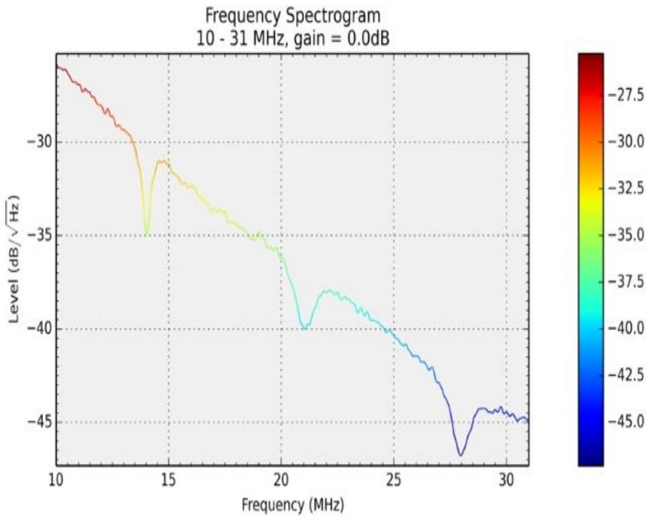
Well it worked after a fashion but of course, that fall off in signal level is due to the zener noise dropping off as frequency increases.
