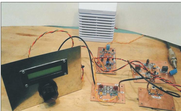
Figure 8—The finished direct conversion receiver.
