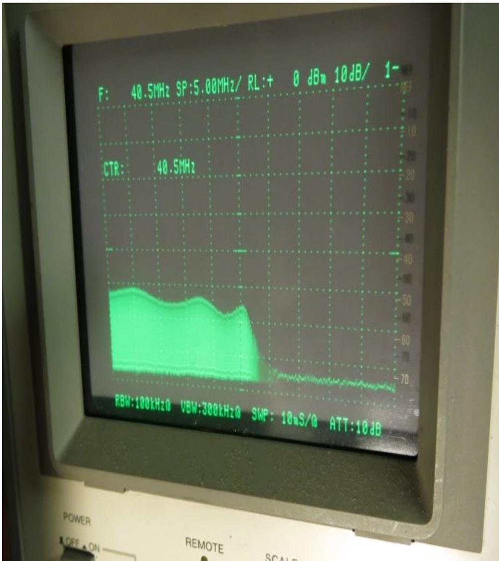
Clearly there is ripple and the cut-off comes a little higher than I would like - but the low pass filter can definitely be seen to be working and I can now make final adjustments to the filter.
