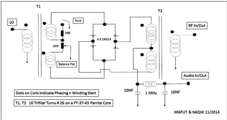
Figure 3—Double balanced mixer schematic.
