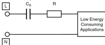
In this case the capacitors are connected in series with the application to the mains and now the functions to be fulfilled are:
