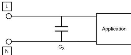
Several functions are combined in these small components: Excellent high frequency properties for short circuiting radio interference, being continuously stressed by the AC mains voltage and not at least having the ability to sustain transient voltages, caused by for example lightning strikes, switching, superimposed on this line.
