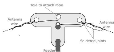
*Strictly speaking a balun should be used but it is often omitted especially for receiving applications. The dipole centre (and don't forget the hose TEE piece dipole centre trick shown in Hot Iron #106!) will also provide a means of attaching a rope to enable the pulley system to hoist the antenna centre. A good quality centre should be used wherever possible (readers of Hot Iron #106 might recall I suggested a plastic hose TEE piece filled with*
