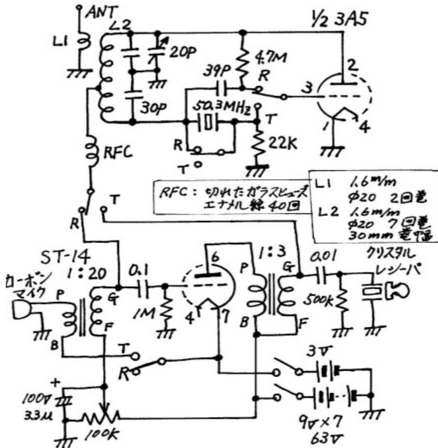
Note how the oscillator / PA is switched to become a regen receiver; not truly bidirectional, but a clever use of the stage in two different “directions”.
