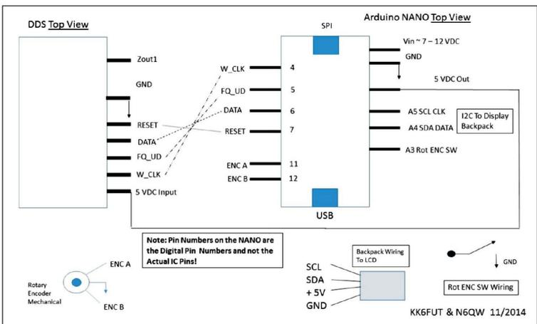
Figure 4—Arduino DDS schematic.
