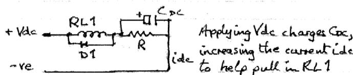
D1 shunts the coil "back EMF" (but delays drop out).
