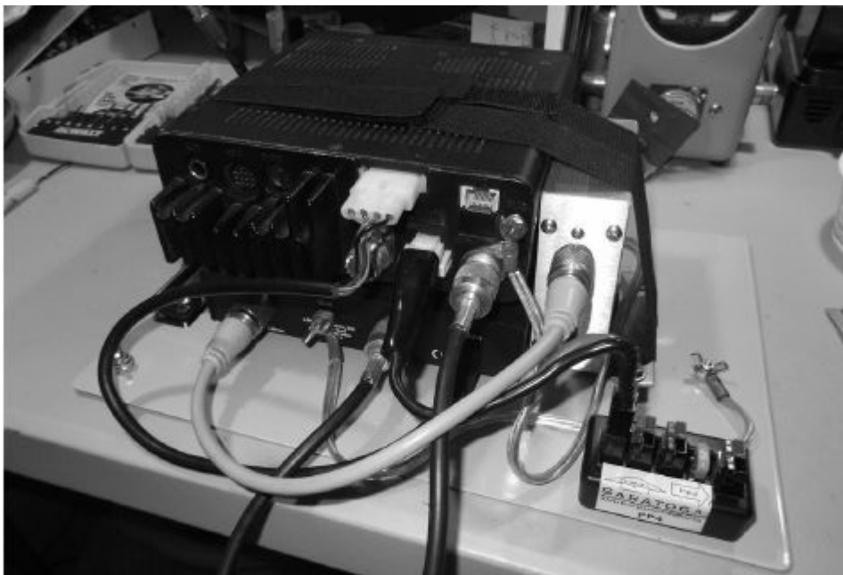
Figure 6.22 — A portable station with a transceiver, antenna tuner, SWR sensing unit, and dc power distribution strip. The equipment is mounted on an aluminum clipboard using heavy hook-and-loop strap. All equipment is bonded to the clipboard with heavy wire jumpers. If installed in the author's vehicle, a ground jumper from the vehicle frame attaches to the wingnut terminals. The entire package can be removed from the vehicle for portable operation, as well.
