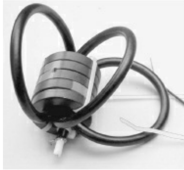
Figure 5.9 — (A) RF choke balun formed by coiling the feed line at the point of connection to the antenna. (B) Ferrite choke balun made by winding coax through a ferrite core. The chokes help isolate the outer surface of the feed line by blocking RF current. The ferrite choke is the preferred method of constructing feed line choke baluns.”
