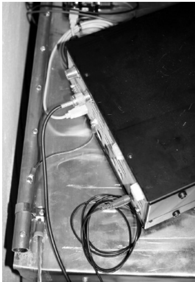
Figure 5.6 — Colling up extra cable length and laying the cable directly on an RF ground plane minimizes the amount of RF picked up by the cable.
