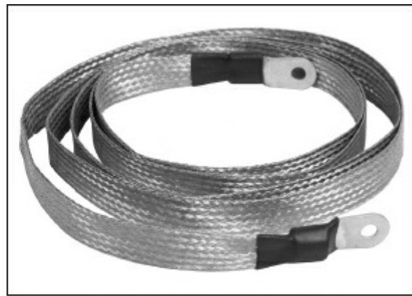
Solid copper strap (A) is the recommended material for grounding and bonding connection at RF. Flat-weave tinned braid (B) can be used if protected from water and corrosive gases or liquids. [Photos courtesy DX Engineering]
