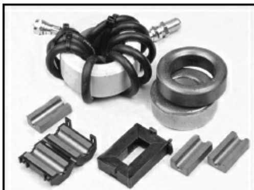
Figure 5.11 — A common-mode RF choke wound on a toroid core is shown at top left. Several styles of ferrite cores for common-mode chokes are also shown.
