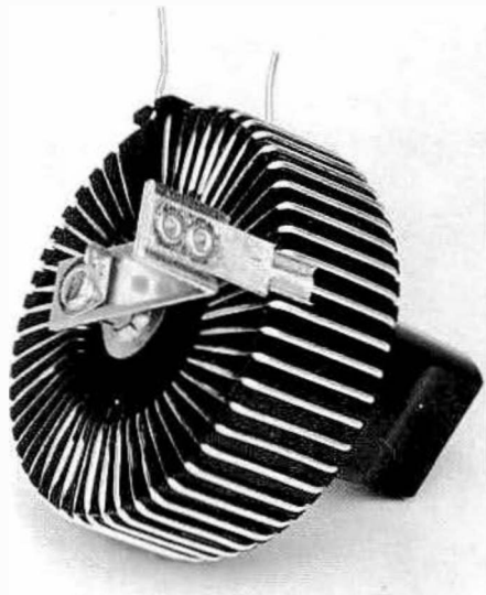
Figure 3-25 Commercially made toroidal type of variable inductor. This unit is manufactured by Ten Tec Corp. for use in their antenna Transmatch. The wiper is built so that it contacts one wire turn at a time, thereby preventing the shorted-turn effect.
