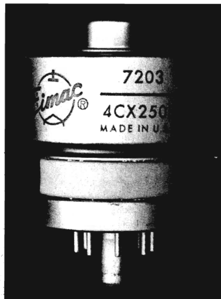
The well known 4CX250B—rated to 500 MHz.
