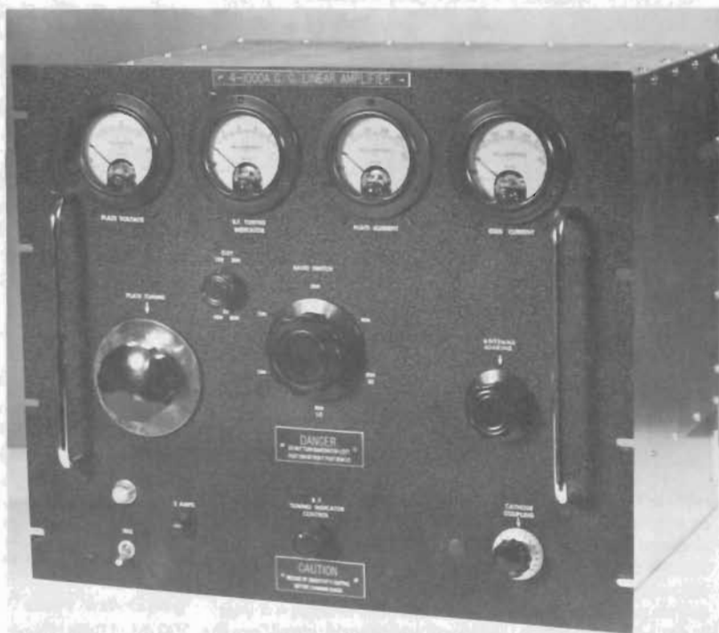
Fig. 1—K9LKA's kilowatt 4-1000A grounded-grid amplifier. Meters across the top of the panel are, from left to right, for plate voltage, relative r.f. output, plate current and grid current. The band-switch control is in the center, flanked by the plate tuning control and capacitor switch S_2 on the left, and the output loading control on the right. Along the bottom are the filament switch, panel lamp and fuse; r.f.-indicator sensitivity control, and the input tuning control.
