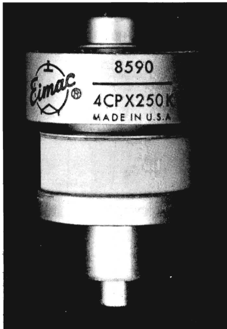
Tube designed for large phased-array radar system. Two of these tubes were used in the 1000-watt 432-MHz amplifier used by WA6LET with a 150-foot dish for moonbounce contacts in 1965.
