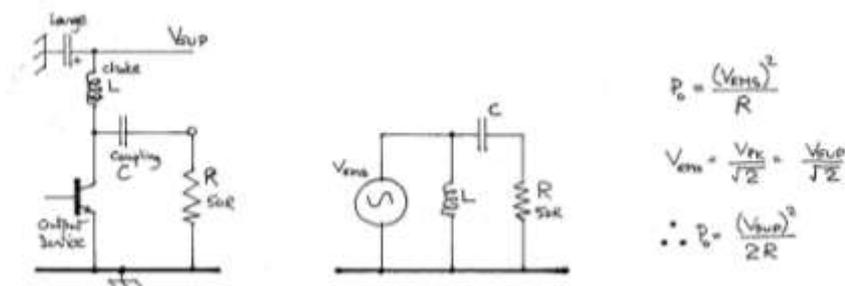
For higher powers, the load on the output device has to be lower – for example, a 5W rig will need a 12.5R load on the transistor when used on 12 volts. Often this is done with a 1:2 turns ratio RF transformer that will perform the four times impedance step up to 50R. Now the supply choke (or inductive reactance of the transformer primary) needs be larger than 50R. G3PCJ
