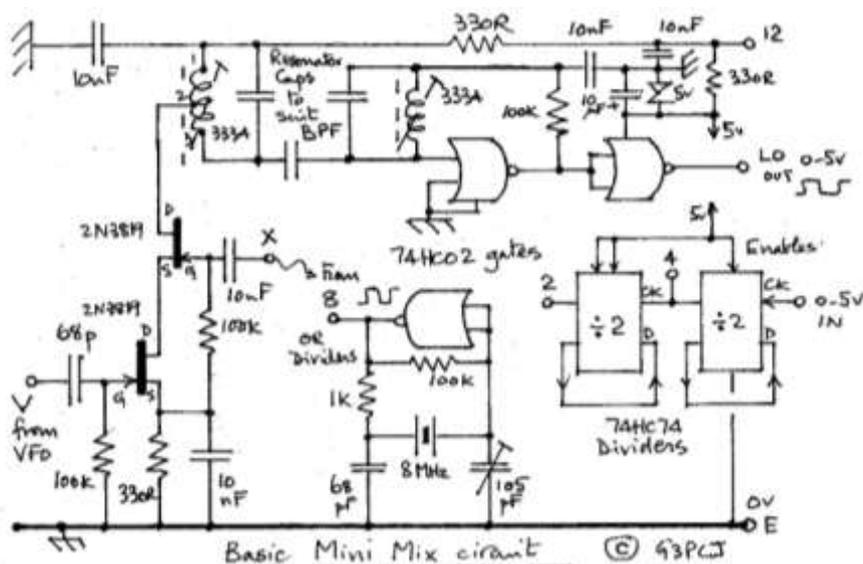
tuned filter (top of PCB) to be used for selection of either the sum or difference signal. To improve its versatility, the middle chip is a pair of digital dividers which can be arranged to divide either the crystal or the output by 2 or 4. This allows a 6 MHz VFO to be mixed with 8 MHz from a crystal to provide 14 MHz, then squared up & divided for 20, 40 and 80m. G3PCJ
