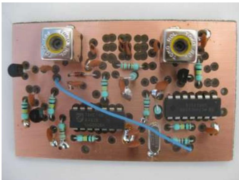
Although this type of mixer is not balanced for either input, it can perform well where the desired output is well removed in a frequency sense from the two inputs; this allows a double
