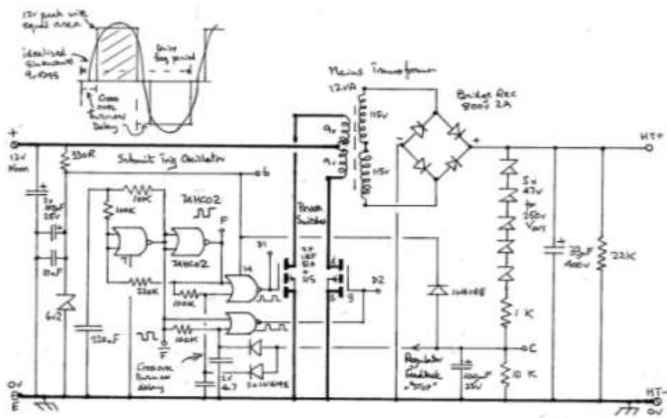
FIG : CIRCUIT OF HT PSU - Take Care - High Voltages! Set Av = 20000 G3PCJ 2/17/15
