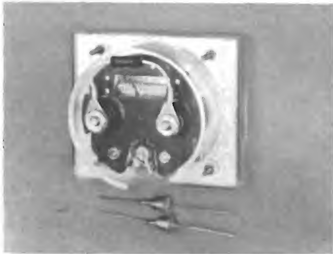
Fig. 1. Diode meter protector connects directly across meter terminals. Unit shown contains two diodes in one package. Silicon top-hat rectifiers shown below are also usable as effective meter protectors after selection by simple tests.
