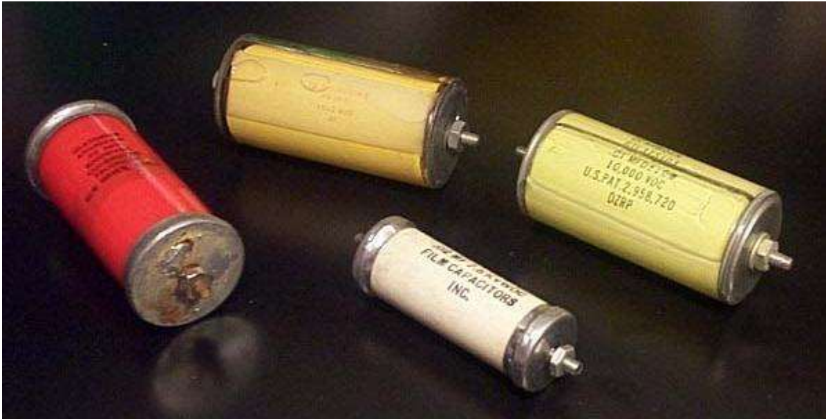
Fig. 9 Suitable Oil-Filled Resonance Capacitors
