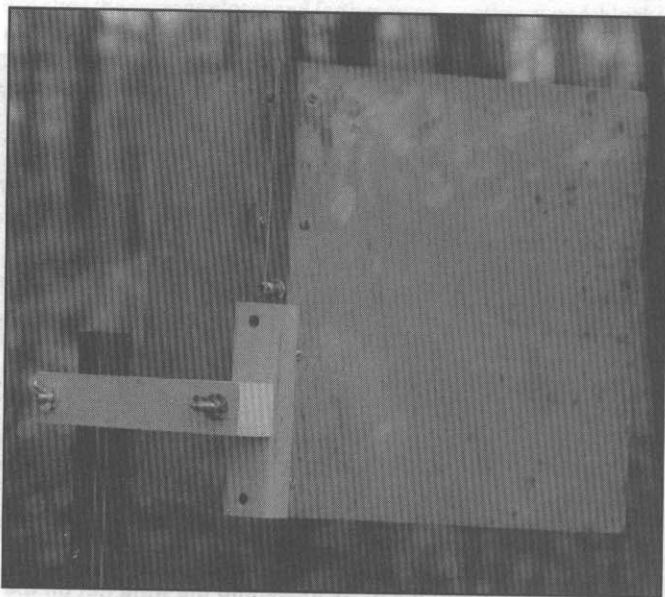
Fig 1—This view of the 900 MHz corner reflector shows the construction from the back side of the antenna.
