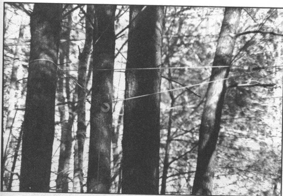
Fig 2—Pulley system mounted on the northwest tree.
