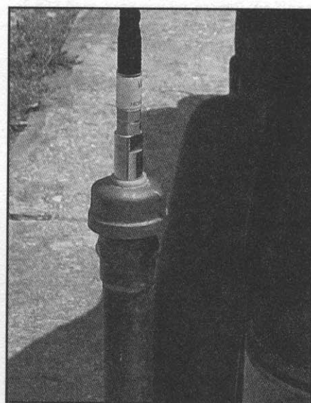
Fig 5—A 1-inch female threaded brass pipe cap with a 1-inch male threaded-pipe-to-copper-pipe adapter. The center of the brass pipe cap was filed to provide a flat surface for the RadioShack antenna mount.
