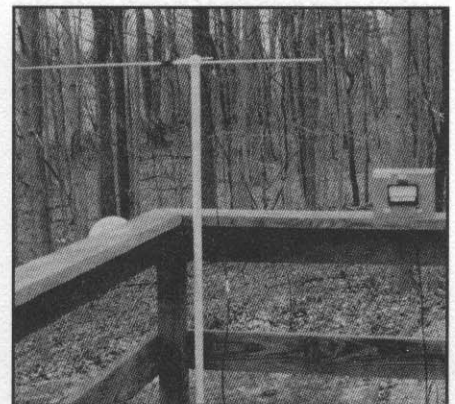
Fig 7—The power meter and dipole antenna setup used for field-strength measurements.
