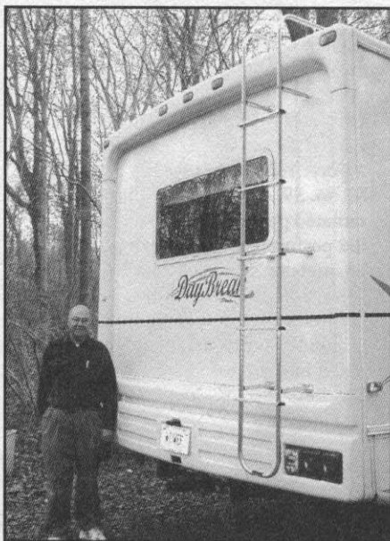
Fig 1—Photograph of W1WEF standing next to his Class-A motor home. The ladder at the back is the stealth antenna.
