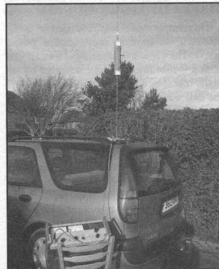
Fig 3—Impedance measurements of a mag-mounted Texas Bugcatcher, using a Hewlett-Packard HP4085A Vector-Impedance meter. I made the measurement with the test probe fixed directly at the base of the antenna—no feeder was used.
