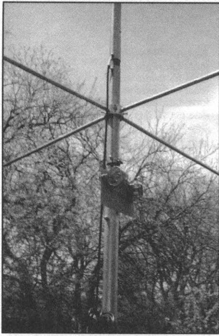
Fig 3—View of the top of the base-mounting section and antenna base, showing the 80-meter network.
