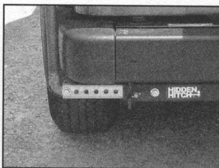
Fig 4—An L made of 1-inch copper pipe inserted and bolted to the 1 \frac{3}{4} -inch square steel tubing bolted through the hitch cross member. Steel tubing is approximately 22 inches long.
