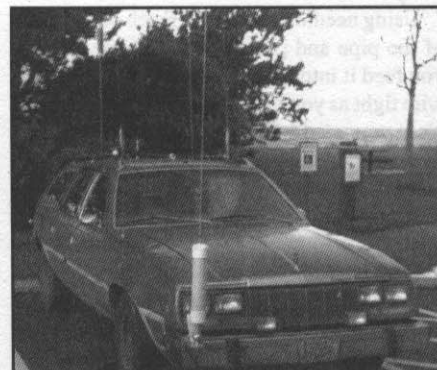
Fig 3—KA7QOR's car, with 160-meter resonator system mounted on front bumper.
