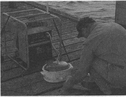
Fig 5—We tied the generator down to keep it from vibrating itself off the pier. The crock pot provided a steady load for the generator and good chow for the operating crew. W5ACS is a good camp cook.
