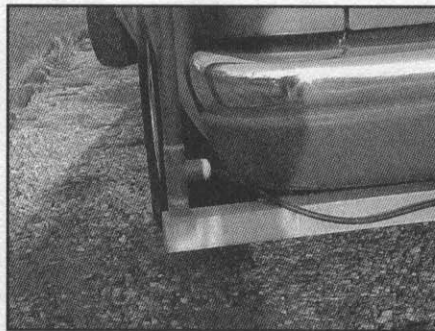
Fig 1—The 1-inch copper T, 1-inch copper pipe and the 2x2-inch square tubing. The coax and the rubber crutch tip are also shown.
