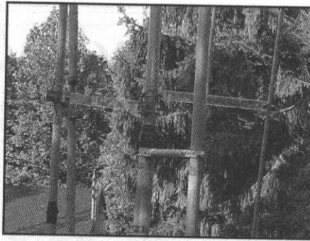
Fig 4—The Plexiglas insulating brackets from the parasitic elements to the center 40-meter element. I've used this antenna successfully on all bands, although the bandwidth on 10 meters is limited to about 200 kHz.
