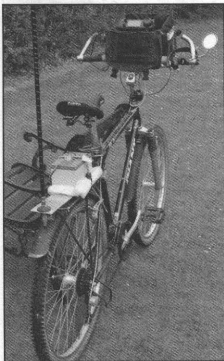
Fig 15—The G3LDO/M HF bike mobile. The rig is located in a handlebar-mounted bag, which gives good weather protection for the radio and provides stowage for the key, headset and logbook. I fixed a thick aluminum plate to the rear carrier to provide a place to fit the battery and a mounting point for the antenna.
