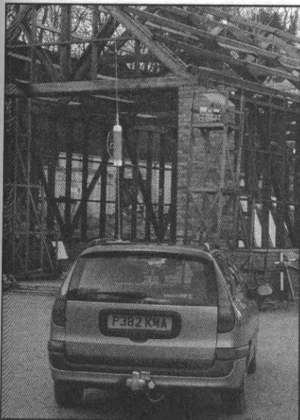
Fig 4—Field-strength measuring arrangement. Most of the antenna measurements were made using a mag-mounted Texas Bugcatcher, the same arrangement shown in Fig 3. Various items of test equipment were tried. In this photo I am using a test instrument known as Hetrodyne Voltmeter type 2002, made in Denmark. I placed this on a wooden mobile scaffolding used for building construction.
