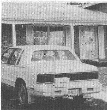
Fig 1 —Photo showing antenna coupler and test antenna mounted on the author's car. The insulated lower section braces the antenna. A 6-inch cord and hook is used to hold the antenna in the lowered position.
