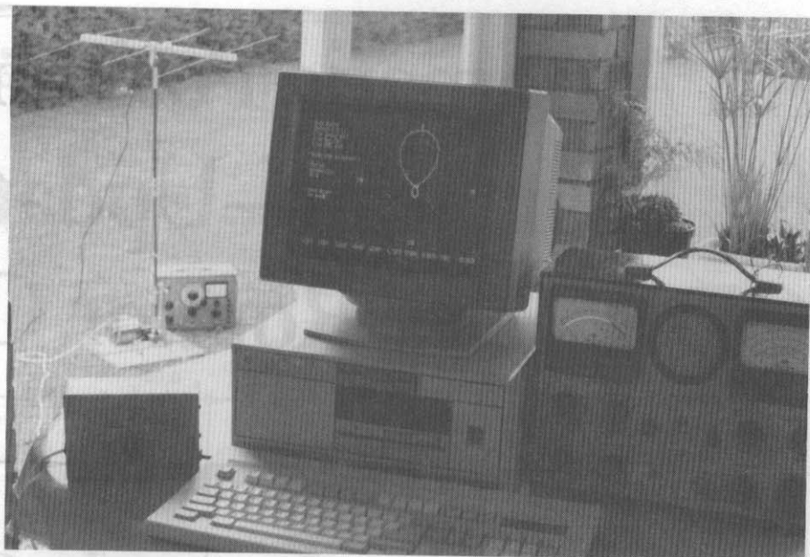
Fig. 7—Photo of IBM-compatible computer with 3-element beam displayed on the monitor. To the left of the computer is the AUT control box and on the right a commercial FSM. The AUT, rotator and signal generator can be seen through the open window.
