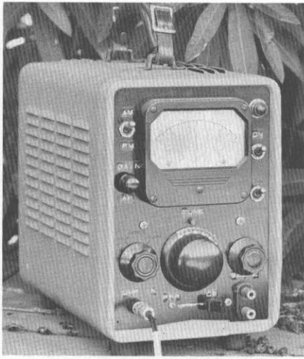
Fig 3—An old HP-415 has become a fully metered UHF telemetry receiver. Knobs on each side of main tuning dial provide meter-range switching and full-scale adjustment. The small knob to the left of the meter controls audio gain. The switch below the tuning dial selects the CW, MCW or PRR inputs.
