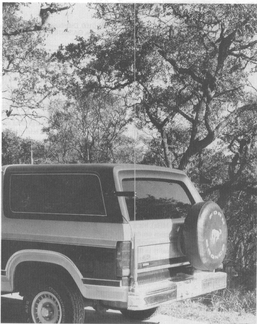
Fig 1—The streamlined mobile whip mounted on a Ford Bronco.
