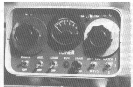
Fig 10—The remote control unit is mounted in a small LMB cabinet. The meter reads antenna current at 1 or 10 amperes full scale. Standard 270° pots with calibrated knobs were used here. These were later replaced with ten-turn pots and counter dials to improve repeatability. The ANT. CUR.-SERVO meter switch is not shown on the schematic since it served only passing interest. What shows as a white line between the cabinet and the feet is a T-shaped calibration chart retained by an elastic band. It provides dial settings for frequencies of interest.
