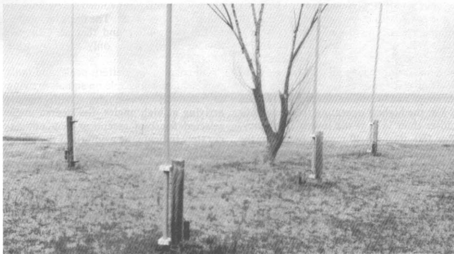
Fig 1—Four of the free-standing antenna elements. The driven element is in the center of the array, near the tree.
