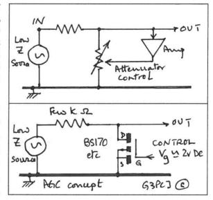
typical output level at the speaker is about 500 mV p-p, and the audio output stage has a voltage gain of x50 (as in LM380-8) then 10 mV p-p is needed from the AFG pot; that might need 40 mV applied to the log pot for a typical setting. Hence the extra control amp needs to produce about 3 volts p-p (allowing for the rectifier to drive the BS170) from an audio input of 40 mV – ie a gain of
