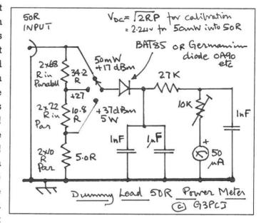
least 50 mA) when producing 2.24v for full scale; this corresponds to 50 mW or 17 dBm (i.e. +17 dB relative to 1 mW into 50R). Use the maths of the previous note! It can then read up to 5W.
