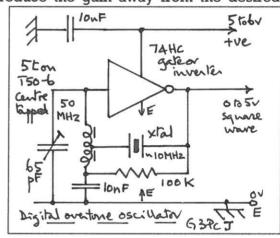
Using this approach in a 'digital' CW TX is straight forward (again with good layout)! One quad NOR gate of a 74HC02 can be the oscillator, with the other three driving a pair of BS170 MOSFETs, it will produce just over a Watt on 6m. The twin pi half wave filter gets rid of any harmonics and you could even contemplate amplitude modulation if that takes your fancy. The main parts of a CW TX are shown below but I leave the TR and sidetone for your creation!
