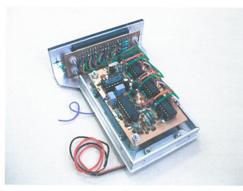
The module can be screened if required, by fitting aluminium sides to the angle sections, with the top screening completed by the transceiver case, forming a box. Only three wires connect the module. The input wire, which when installed will be about 40mm in length, plus the two wires for power and ground. The display works very well, and I hope to give a further report on overall progress of the transceiver in due course. MOGWD
