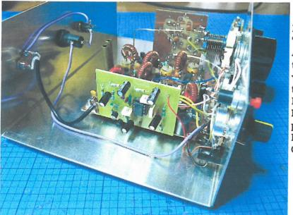
Here is another Berrow built by Philip Thompson G4JVF, this time with the AGC kit nearest camera and what I think might be a keyer beyond the air variable. This is the one that has been tried on all four of its normal 20 - 80m bands! It also has the two chimney heat sinks! I am awaiting Philip's reports of experiments with higher bands when he has nothing else to do! G3PCI
