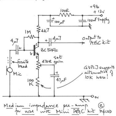
speech clipper but will not over-modulate. Users of high output fist microphones might find that a 4K7 preset would be better so the gain can be further reduced if necessary. One could also try feeding the audio from the AGC kit (with or without pre-amp as necessary) into a speech processor so as to raise the average speech level closer to the peak level and thus increase 'talk power'!
