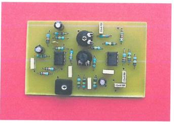
The kit is normally connected immediately before the rig's main audio gain control stage – either automatic or manual. It can also be used as a separate receiving accessory outboard of an existing rig to drive medium Z phones. Apart from the optional frequency control, the other front panel items are the frequency range and notch/peak toggle switches. The PCB is single sided (50 x 80 mm) and needs a 9 to 22 volt supply. Cost is £18.
