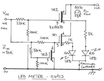
TR3 then comes on at about 8 volts, acting as a switch across the input to TR1 so that only the red LED is left on! I have to admit that I have not tried this out but I am reasonably confident it will work - maybe with some resistor value alterations!
