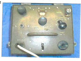
**Type D Wavemeter** spot frequencies 1.9 - 8.0Mc/s in two ranges. The gaps filled by VFO (centre knob) with 1 MHz pips to 25Mc/s. Worked off 6Volt cell
