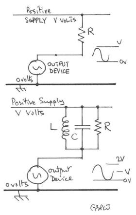
which is sitting on a DC pedestal of V volts also! Practical output networks remove the DC aspect by capacitive coupling so that the we are now only concerned with an ac signal of amplitude V volts peak into the load resistance R.
