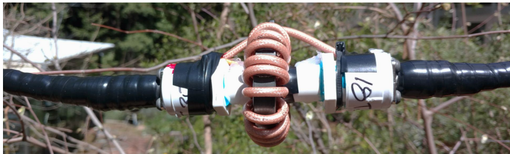
Fig 12 – W6GJB's Inline Chokes
