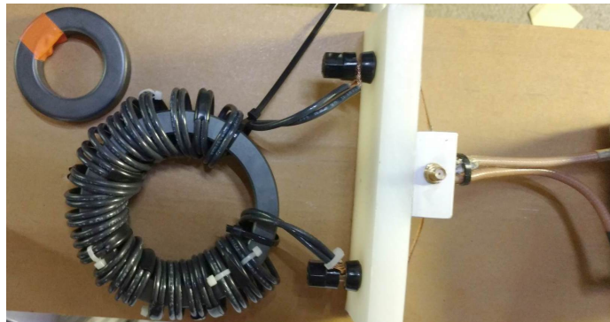
4-in o.d. THHN Choke In Test Fixture
