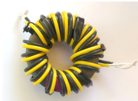
Fig 9 – A Teflon Choke
